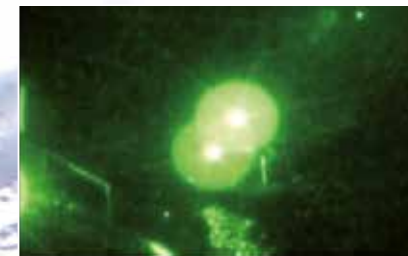
Image intensification: image is saturated by looking directly at a light source.
